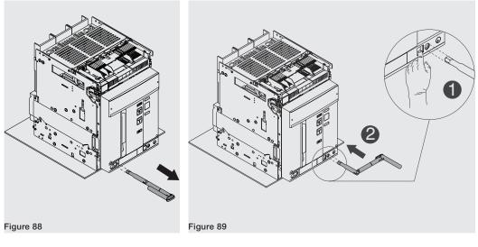
10. Turn the crank clockwise until the pushbutton comes out and the indicator shows that the circuitbreaker is in TEST position. See Figure 90.
