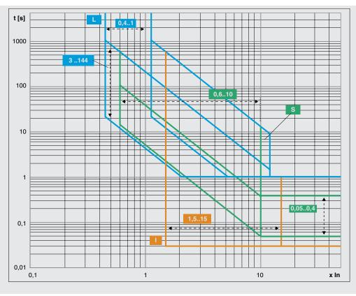
Tripping curve for L-S(t = k)-I protections
