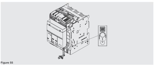
7. Press the lock button and then rotate the crank clockwise until the button comes out and the indicator shows that the circuit-breaker is in the **CONNECT** position. See Figure 56.
