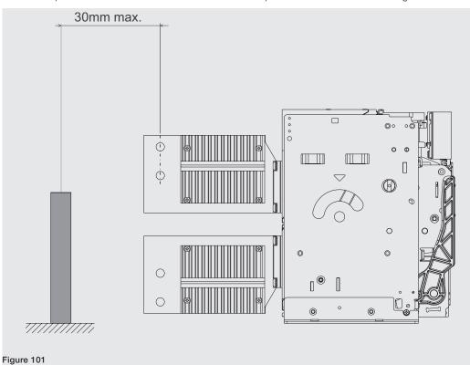
>690V version circuit-breakers Insulating protections must be assembled for >690V circuit-breakers as indicated in the figure.
