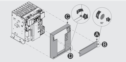
Figure 114 - Removing the flange and front cover
