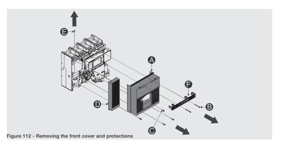
After reassembling the accessories, the parts previously dismantled must be reassembled as indicated:
