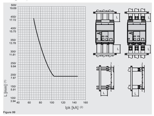
(1): distance of the first anchor plate from the circuit-breaker terminals(2): peak current
