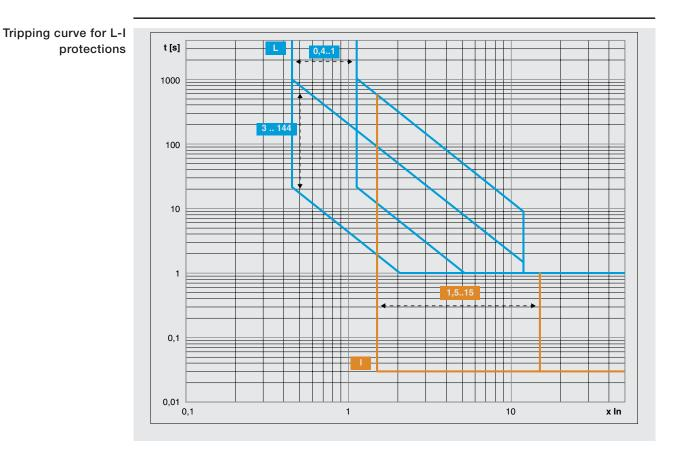
The following are the trip curves of the protections available with Ekip Dip trip units.
