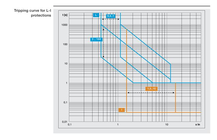
Tripping curve for L-S(t = k / I <sup>2</sup>)-I protections
