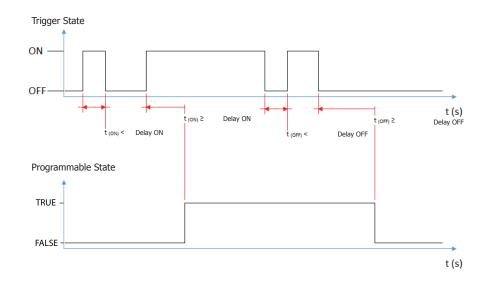
The states can be used with the external Ekip Signalling 10K module, on Link Bus or with the programmable functions, to transfer the desired signalling combination on contacts.
