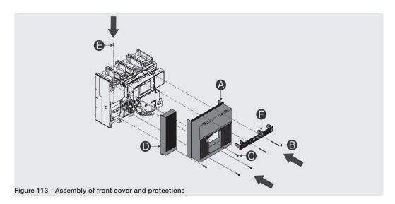
Disassembly operations for To dismantle the accessories, the following parts must be removed from the circuit-breaker:
