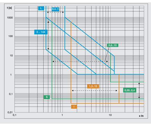
Tripping curves for protection L according to IEC 60255
