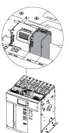
Termination resistor The modules provide the possibility to insert a 120  $\Omega$  termination resistor on the CAN bus, by setting the dipswitches Rterm on the side of the modules, in position on. This option must be selected before the modules are installed.
