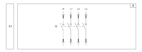
Diagram B - General diagram of the switch-disconnector
