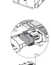
Termination resistors The modules provide the possibility to insert a 220  $\Omega$  termination resistor on the RS-485 bus, by setting the dip-switches Rterm on the side of the modules, in position on.
