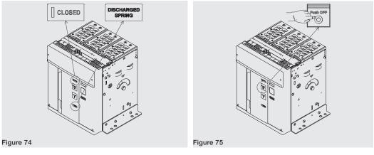
7. Check that the circuit-breaker is open (open / closed indicator "O - OPEN"), and check that the springs are discharged (spring signalling device "white - DISCHARGED SPRING") as indicated in Figure 76.
