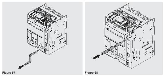
To extract the moving part from the fixed part, perform the same steps indicated for insertion in reverse order. After extraction, in order to remove the moving part, unlock the safety lock. See Figure 59.
