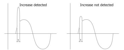
The alarm threshold available in the menu, **V Spike Threshold**, is expressed as %Un.
