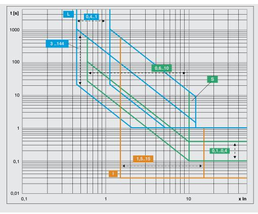
Tripping curve for L-S(t = k)-I protections
