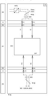
Diagram 31 - Direct auxiliary power supply
