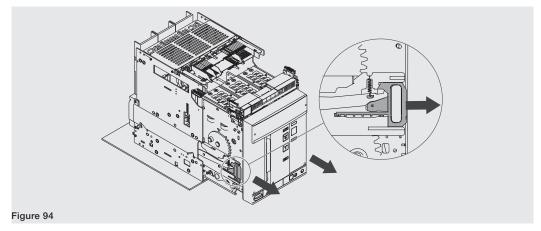
Always use both levers of the guides on the fixed part when racking out the circuit-breaker. See Figure 94.
