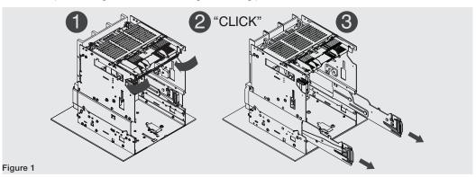
2. Position the lifting plates on the mobile part making sure that the tongue of the plates is latched properly. See Figure 82.
