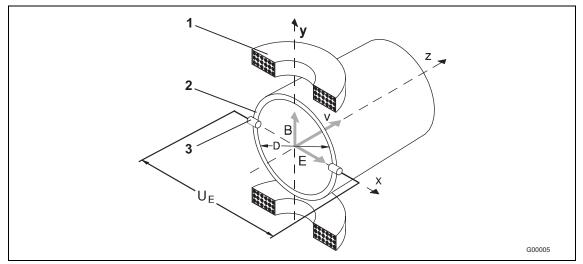
Fig. 4: Electromagnetic flowmeter schematic
