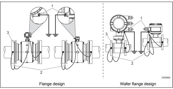
Fig. 27: Plastic pipes, non-metallic pipes or pipes with insulating liner
