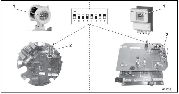
Fig. 56: Position of DIP switches
