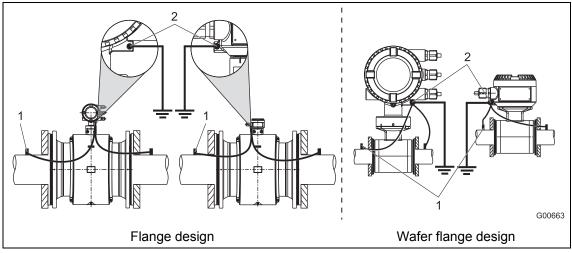
Fig. 26: Metal pipe, without liner
