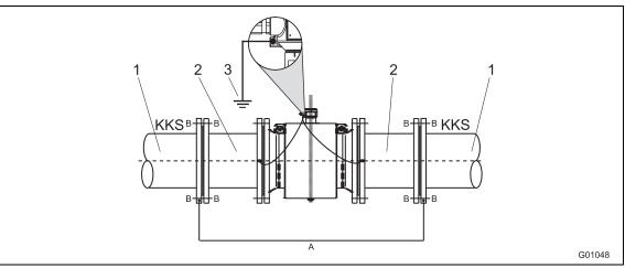
Fig. 31: Flowmeter sensor with functional ground
