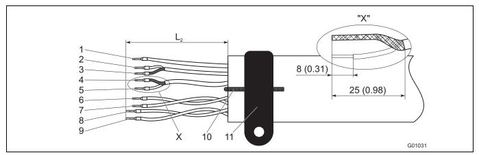
Fig. 35: Transmitter side, dimensions in mm (inch)
