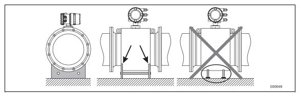
Fig. 9: Support for meter sizes larger than DN 400
