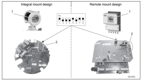
Fig. 55: Position of DIP switches
