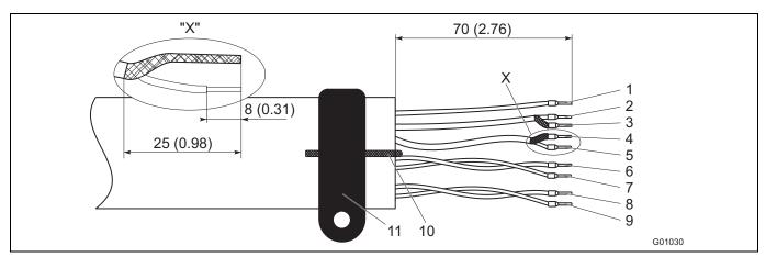
Fig. 34: Flowmeter sensor side, dimensions in mm (inch)
