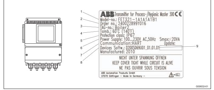
Fig. 3: External transmitter (remote design)
