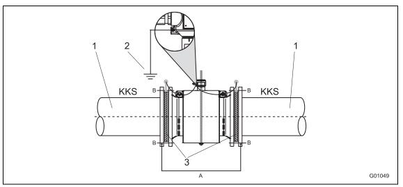
Fig. 30: Flowmeter sensor with grounding plate and functional ground
