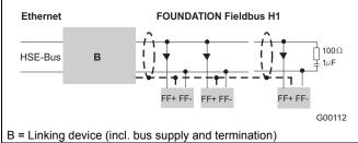
Fig. 53: Example for FOUNDATION Fieldbus interface connection
