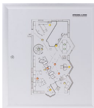
Example control panel with layout and control lights (delivery unprinted/ not wired)
