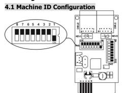
There are eight bits to present ID of each card. Use SW1 to set machine ID. From left to right, it's 8 to 1. As shown, when the switch is pushed down, the bit is set to "one". Otherwise, the bit is set as zero. The ID of modbus card is set to 0x01 as chart. Please check appendix for detailed ID no. and SW1 setting.
