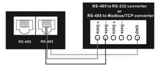
Wiring connection between RJ45 and media converter
