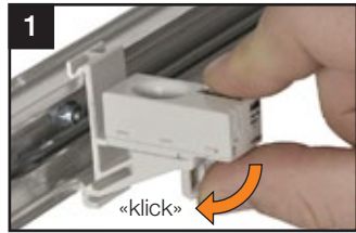
"Click" device on DIN rail
