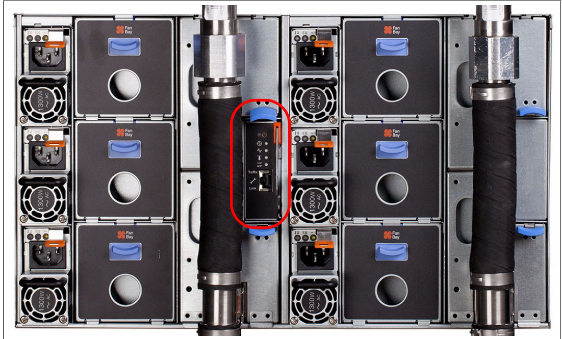
Figure 3-8 Rear view of the chassis that shows the location of the FPC
