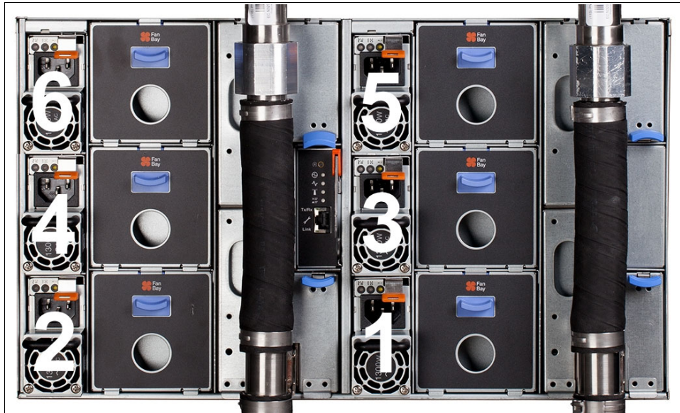
Figure 3-4 NeXtScale n1200 WCT Enclosure rear view with power supply numbering
