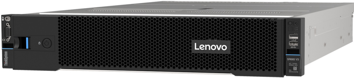
Figure 26. Lockable front security bezel
