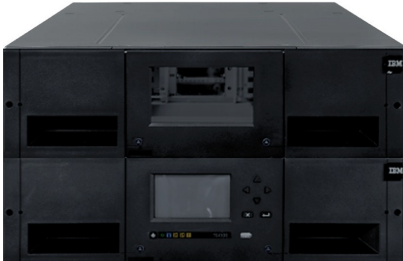
Figure 1. IBM TS4300 Tape Library: Base module (bottom) with one expansion module (top)
