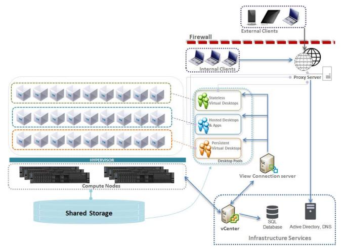
Figure 1: LCV reference architecture with VMware Horizon
