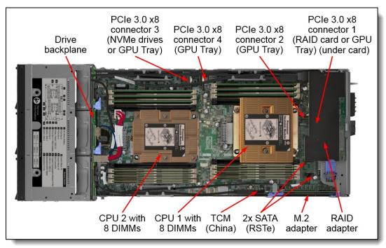
The following figure shows the internals of the SD530 server identifying key components.
