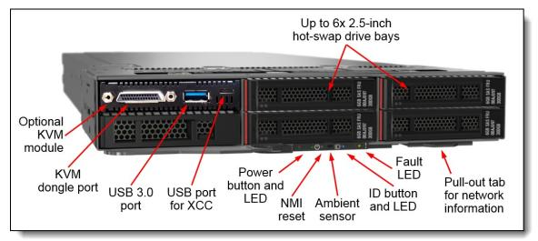
Figure 5. Front view of the SD530 compute node
