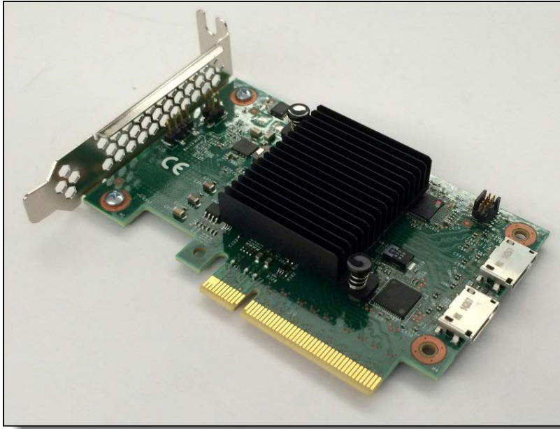
Figure 7. NVMe PCIe SSD Extender Adapter
