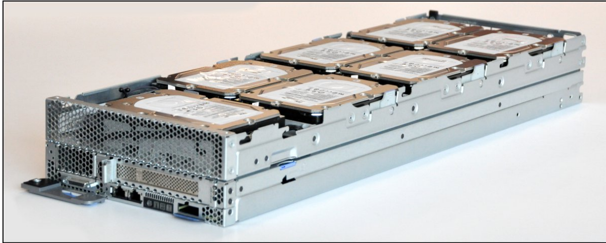
Figure 6. NeXtScale 12G Storage Native Expansion Tray attached to an nx360 M5 compute node
