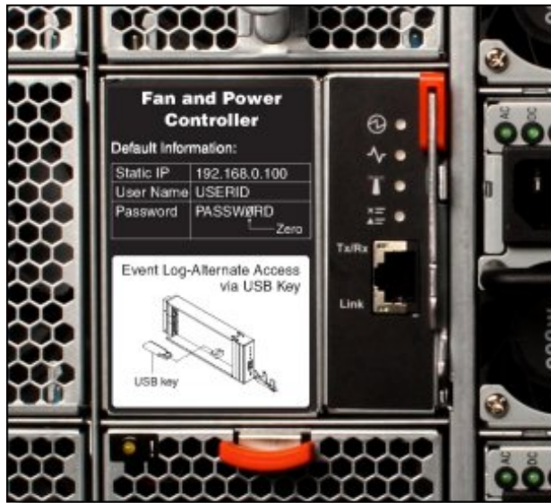
Figure 18. Fan and Power Controller
