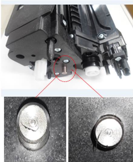
Imaging Unit's cleaning & checking point
