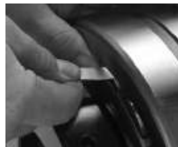
Fig. 18. Measure RIC before installation.
