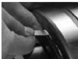
Fig. 14. Measure RIC before installation.
