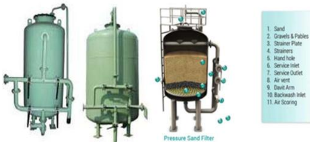
Fig 7.5 Pressure Sand Filter
