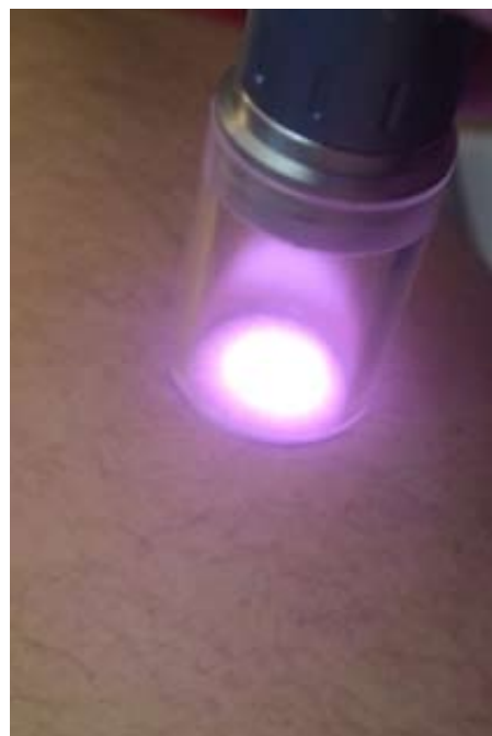
Figure 2. Class IV Lasers use infrared wavelengths which are invisible, but can be photographed with a digital camera.
