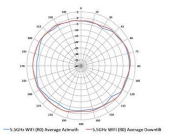
5.5GHz Wi-Fi (dual-radio mode, radio 0)
