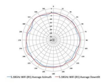
5.18GHz Wi-Fi (dual-5GHz mode, radio 1)
