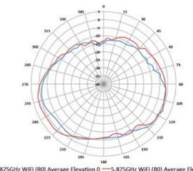
5.875GHz WiFi (R0) Average Elevation 0 -5.875GHz WiFi (R0) Average Elevation 90
