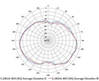
5.18GHz Wi-Fi (dual-5GHz mode, radio 1)
