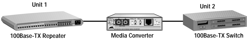
Figure 2 Example of a Duplex Mode Mismatch
