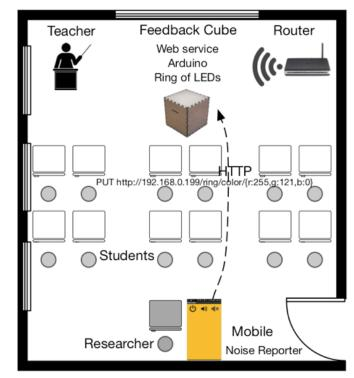
Fig. 2. Technical setup used to deploy the ALD in the classroom.
