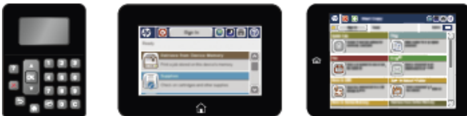
Figure 4-2 FutureSmart 4 control panels
