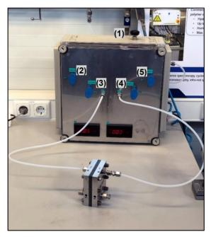
Figure 3.4: Leak checking device, (1) Flow control valve, (2) and (3) Gas input valve, (4) and (5) Gas output valve
