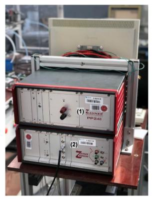
Figure 3.10: EIS electrochemical workstation, (1) Zahner PP241 power potentiostat, (2) Zahner Zennium device.
