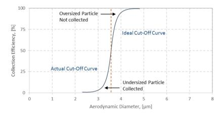
Figure 13: Determination of the cut-off diameter by plotting the collection efficiency curve.
