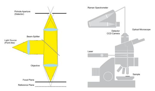
Figure 23: Basic scheme of a confocal microscope and Layout of a confocal Raman Spectrometer.
