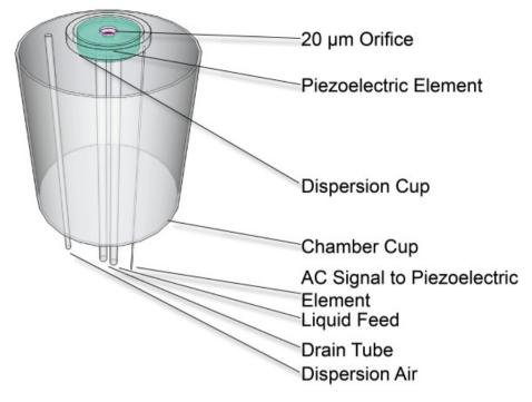
Figure 1: Schematics of the core unit of the vibrating orifice aerosol generator.
