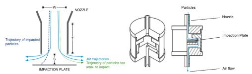
Figure 12: Left: Jet trajectories for an inertial impactor (see Marple et al. (1976) [107]), Right: Schematics of inertial impactor used at SGAS-ESL.
