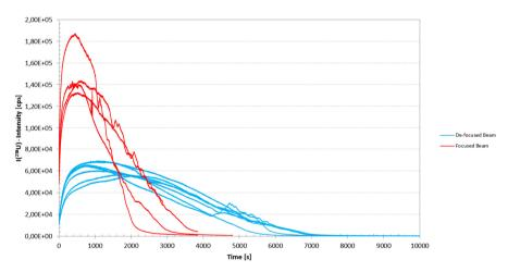
Figure 85: Comparison of focused and de-focused ion beam on the 238U intensity profile.
