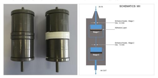
Figure 29: Left: Photo of modified inertial impactor designed at SGAS-ESL; Right: Scheme of MII.
