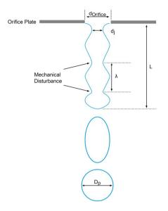
Figure 2: Diagram of liquid jet break up cycle induced by piezo electric disturbance.
