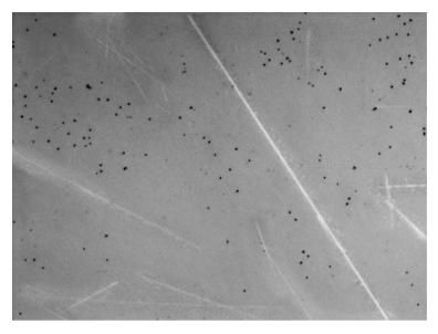
Figure 24: Target surface after vacuum impaction, with visible score marks.
