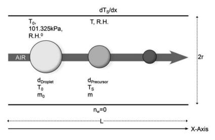
Figure 3: Schematic of spray pyrolysis: evolution of droplet-to-particle conversion in a heated flow reactor.
