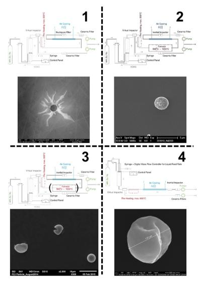
Figure 17: No (1): First setup with neodymium precursor particles (wet); No(2): First fully operational setup to produce dry neodymium oxide particles; No(3) Uranium oxide particles from SG140521\_02; No(4) latest evolution step of the setup as from December 2014.
