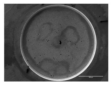
Figure 18: SE-image of a corroded high grade steel orifice used to produce uranium particles.
