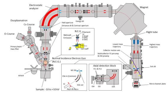
Figure 15: Schematics of Cameca's IMF1280 LG-SIMS, courtesy of CAMECA.
