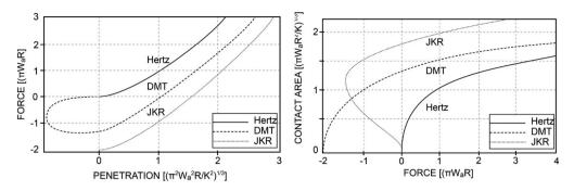
Figure 10: Contact relations for the Hertz-, DMT- and JKR-models.
