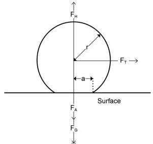
Figure 11: Particle with radius "r" adherent on surface with a contact area "a". Several forces act on the particle including: gravitational force " $F_G$ ", adhesion force " $F_A$ ", external tangential to surface " $F_T$ " and external force normal to surface " $F_N$ ".
