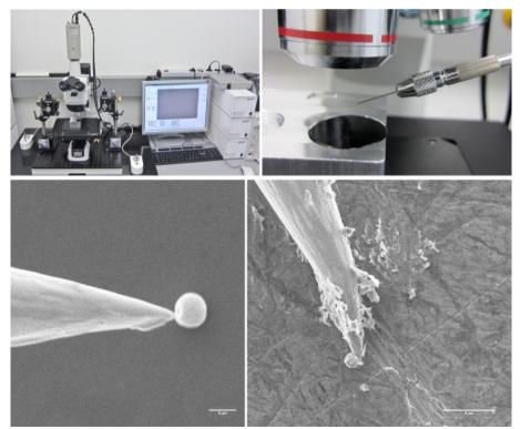
Figure 20: Top: SURUGA-Particle manipulation system at SAL and bottom: SE-images depicting the transfer of single micrometer sized particles, recorded with Jeol JSM 6610.
