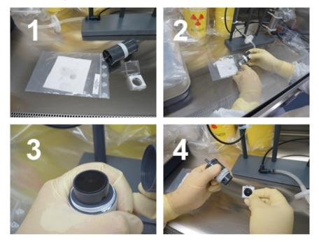
Figure 32: Sequence of sample preparation for µ-Raman measurements.
