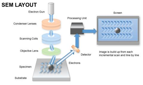
Figure 14: Layout of a Scanning Electron Microscope.
