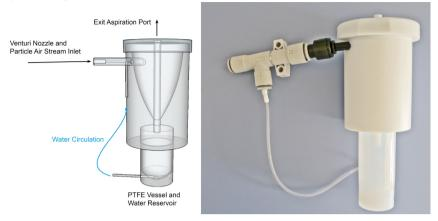
Figure 33: Left: Schematics of Cyclone Sampler with Venturi Nozzle Inlet and right: Image of the Cyclone Sampler with Venturi Nozzle.
