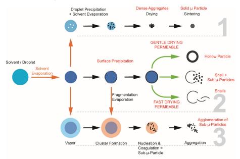
Figure 5: Schematics of droplet-to-particle morphology evolution during thermolysis, see Messing et al. (1993) [58] and Reuge et al. (2008) [66] [67].
