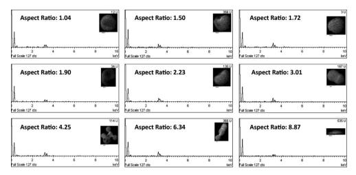
Figure 37: Aspect Ratio deviations due to particle deformations, agglomerations, artefacts and measurement errors.
