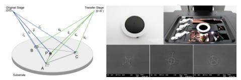
Figure 21: Left: Vector diagram representing the triangulation method. A, B, C are reference marks, P is the particle of interest, O the source instrument and O' the target instrument. (See Admon, et al. 2005 [9]); Right: Reference marks: (left hand side) either by scratching with a tungsten needle or (right hand side) by LMD.
