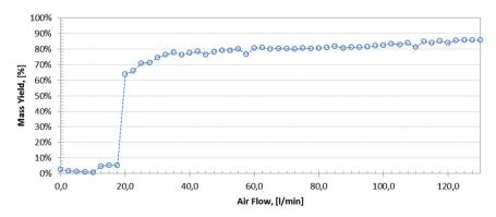
Figure 34: Collection efficiency of the cyclone sampler at various air flows.
