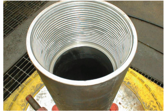
An example of a JFEBEAR coupling where Clear-Plate™ has been applied as the end finish
