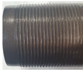
✓ Correct amount of thread compound applied
