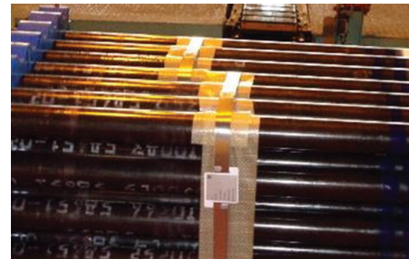
Image 6 – polypropylene overlapping technique
