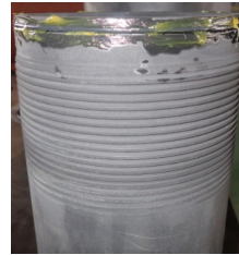
Figure 10.1.3 – O-ring fitted (Plug)
