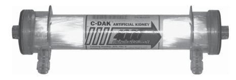
common membrane modules are plate-and-frame devices and hollow-fiber cartridges. Compact hollow-fiber **hemodialyzers**, such as the one shown in Figure 14.13, contain several thousand 200- $\mu$ m-diameter fibers with a wall thickness of 20–30  $\mu$ m and a length of 10–30 cm. Dialysis membranes can be thin because pressures on either side of the membrane are essentially equal. The differential rate of solute mass transfer across the membrane is
