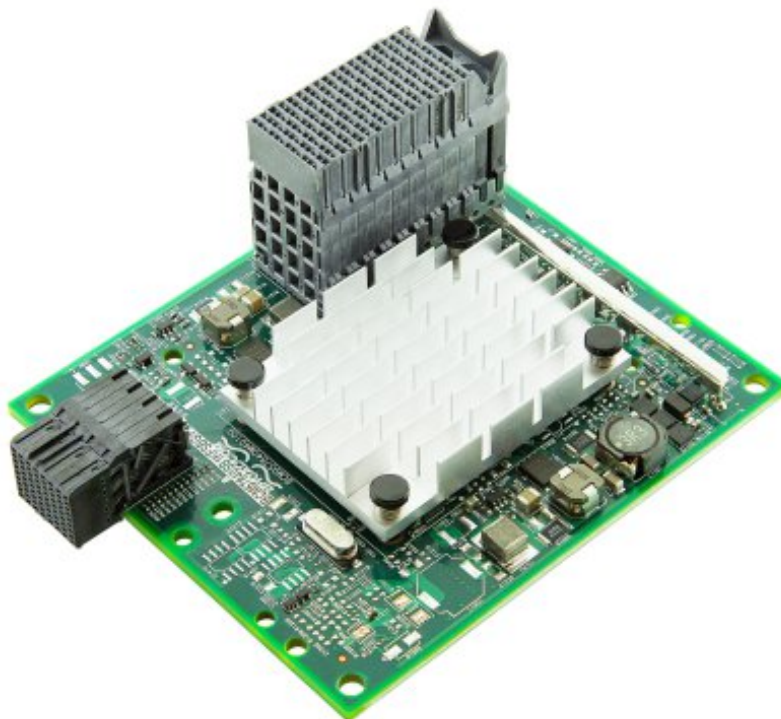
Figure 1. Flex System CN4022 2-port 10Gb Converged Adapter and EN4172 2-port 10Gb Ethernet Adapter
