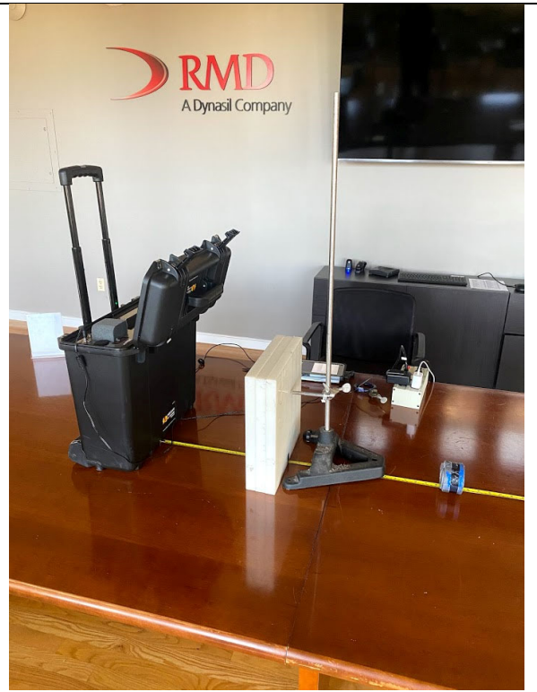
Figure 11b. Moderated Cf-252 measured for 10 minutes at 40 cm away
