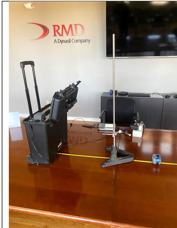
Figure 11a. Bare Cf-252 measured for 10 minutes at 40 cm away
