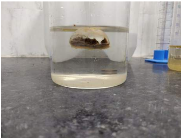
Fig. 4 After the end of decalcification process in 0.6 N HCl, femoral head starts floating in the HCl solution
