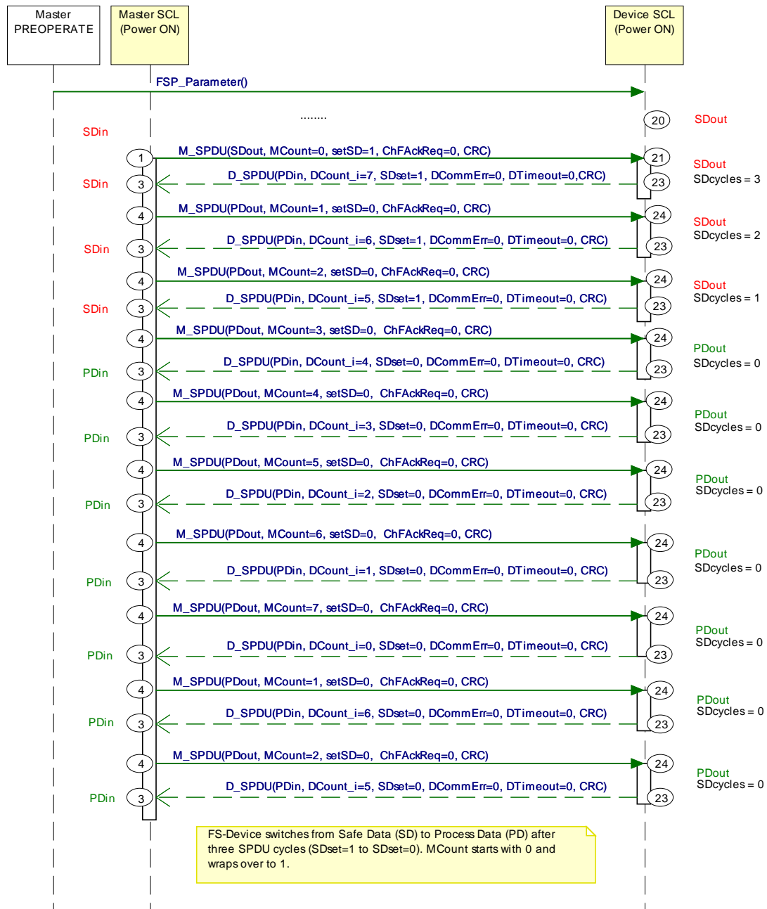
Figure 48 – FS-Master and FS-Device both with power ON
