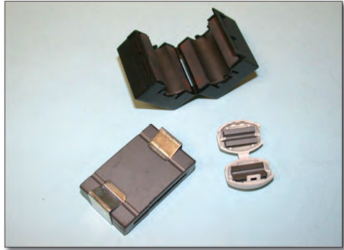
FIGURE 20: Examples of various clamp-on ferrite chokes.
