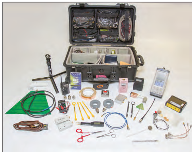
FIGURE 1: Troubleshooting kit with most of the major components shown. The spectrum analyzer is the Thurby Thandar model PSA6005 and tunes from 10 MHz to 6 GHz. Everything fits inside a Pelican 1514 roller transit case. The contents are described in Part 1 and Part 2 of this article.
