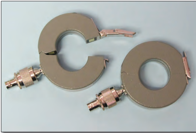
FIGURE 14: A matched set of clamp-on Fischer Custom Communications model F-33-1 current probes. While not imperative to purchase, a matched set is very useful for advanced troubleshooting I/O cable emissions. They can sense RF currents of a few microamps.
