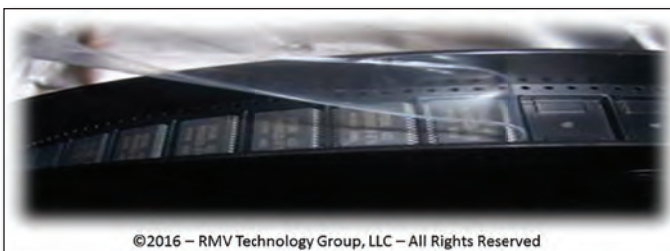
FIGURE 2: Tape and Reel Photograph showing components in carrier tray and clear film
