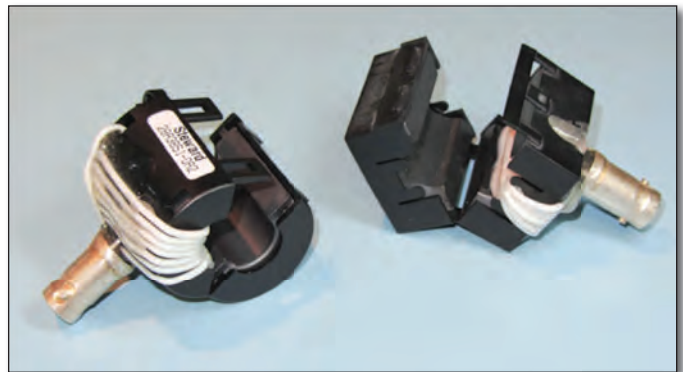
FIGURE 13: An example of simple current probes you can make to measure harmonic RF currents in cables.
