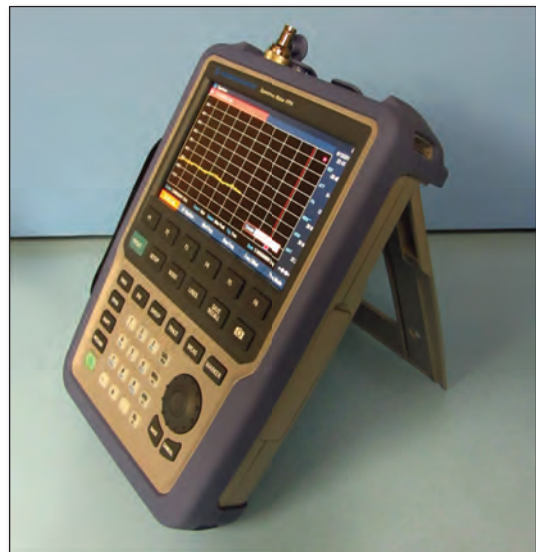
FIGURE 6: The Rohde & Schwarz FPH "Spectrum Rider" portable spectrum analyzer tunes from 5 kHz to 2 GHz or an optional upper limit of 3 or 4 GHz as budgets allow. The specifications are very similar to much higher-priced lab quality analyzers and the base price is just $5,280.
