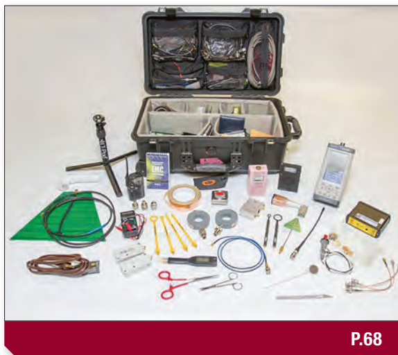
Troubleshooting kit with most of the major components shown. The spectrum analyzer is the Thurlby Thandar model PSA6005 and tunes from 10 MHz to 6 GHz. Everything fits inside a Pelican 1514 roller transit case. The contents are described in Part 1 and Part 2 of this article. (From Assembling A Low Cost EMI Troubleshooting Kit – Part 1 (Radiated Emissions) by Kenneth Wyatt)
