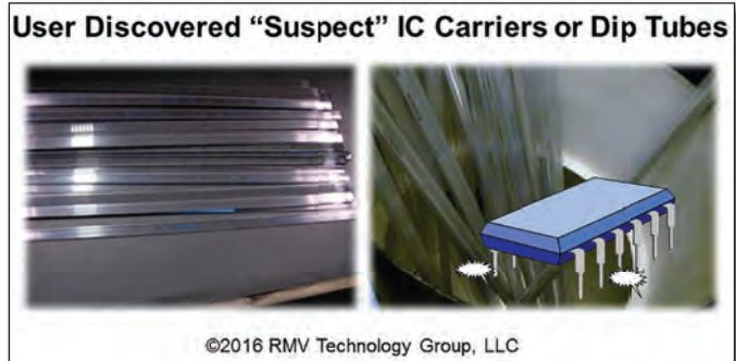
FIGURE 5: IC Carrier or Dip Tubes which were Quarantined by User
