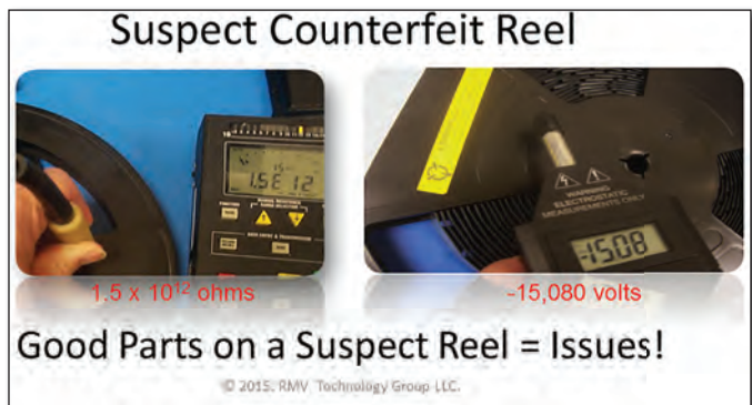
FIGURE 6: 2-Point Resistance Test of Reel on Left and Non-Contact Voltage Reading on Right
