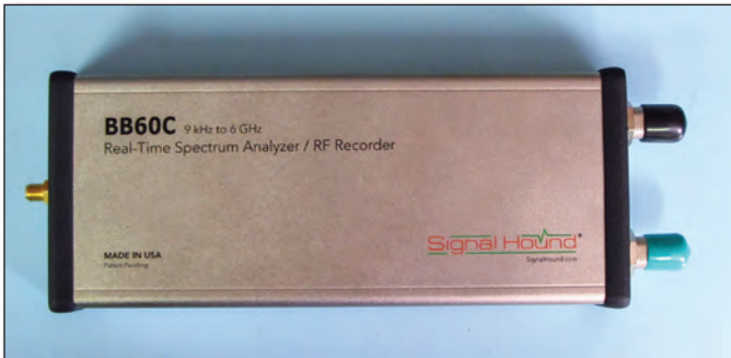
FIGURE 8: The Signal Hound BB60C USB-controlled real-time spectrum analyzer covers 9 kHz to 6 GHz and has a real-time bandwidth of 27 MHz. The cost is $2,879.
