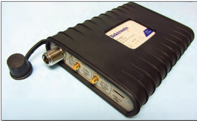
FIGURE 7: The Tektronix RSA306 USB-controlled real-time spectrum analyzer covers 9 kHz to 6.2 GHz and has a real-time bandwidth of 40 MHz. The base cost is $3,489 and there are several digital modulation display options.
