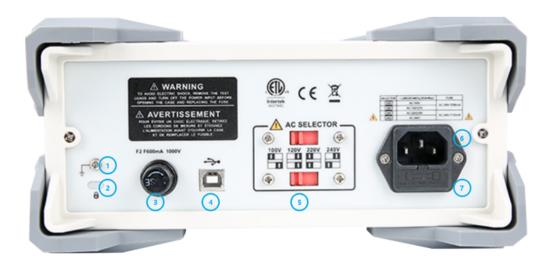
① GND ② Lockhole ③ Current measurement fuse ④ USB Device interface ⑤ AC voltage selector ⑥ Power supply interface ⑦ Power supply fuse
