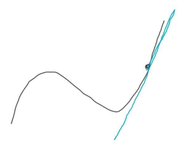
(a) When the function  $\vec{f}(\vec{x}, \vec{y}) : \mathbb{R}^n \times \mathbb{R}^k \to \mathbb{R}^m$  takes in vectors and outputs a vector (rather than a scalar), we can view each dimension in  $\vec{f}$  independently as a separate function  $f_i$ , and linearize each of them:
