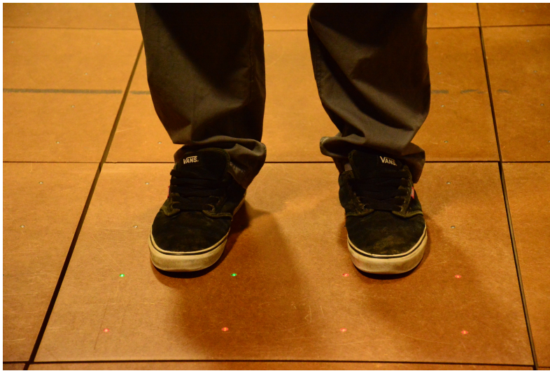
Figure 3.15 – Using the load-sensing tiles as weighing scales. The LEDs encode different units of weight with different colors (red = 10 kg, yellow = 5 kg, green = 1 kg).
