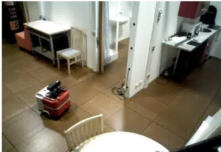
Figure 7.1 – An autonomous robot navigating on a pressure sensing floor.
