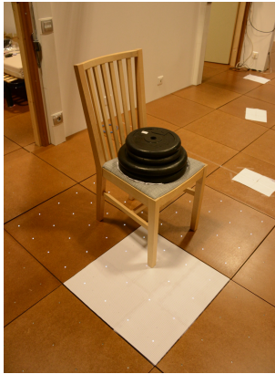
(a) A chair being scanned on a scanner made of 4 load-sensing tiles. One tile was covered in millimeter paper, to be used as a location reference. Translations were performed by hand.
