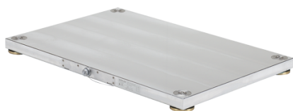
Figure 2.22 – Kistler portable multi-component force plate for 10 kN, Type 9286B [72]
