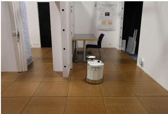
(a) A PekeeII robot on a tiled load-sensing floor with embedded processing units [107]
