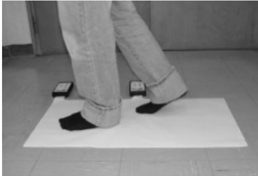
Figure 2.11 – The TechnStorm foot analyzer pressure-sensing mat, employed by Jung et al. in [66].
