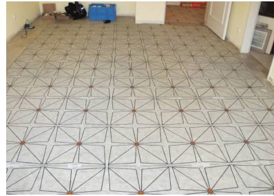
Figure 2.25 – The SensFloor, presented by Lauterbach et al. in [80].
