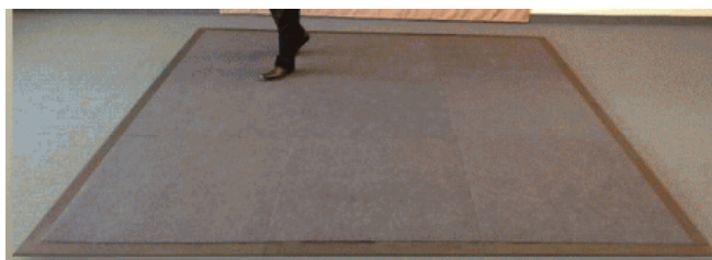
Figure 2.23 – The GAITRite Surface pressure-sensing floor [50]
