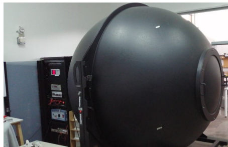
Figure 1: Integrating sphere for luminous flux detection according to IES LM 79
