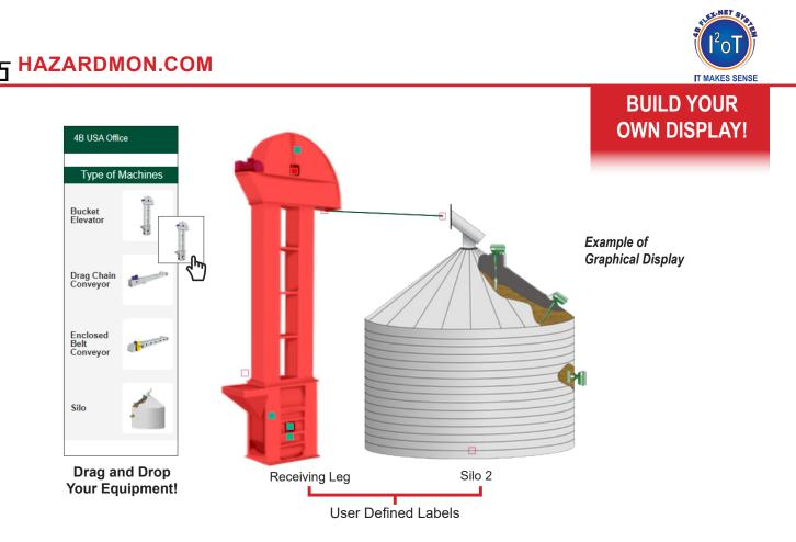
The IE-NODE has in-built network support for Hazardmon.com service connectivity. HazardMon is a secure cloud based hazard monitoring solution providing status notifications and data logging for bucket elevators and conveyors. Live system status, graphs and historical data can be viewed on any web-enabled device (smartphone, tablet PC, desktop or laptop computer).
