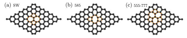
Figure 1: Three structural defects in graphene: (a) Stone-Wales, (b) Divacancy 585, and (c) Divacancy 555-777
