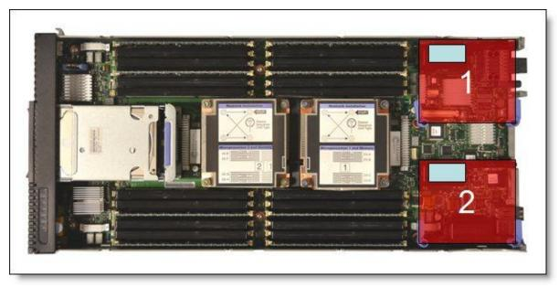
Figure 6. Location of the I/O adapter slots in the IBM Flex System x240 Compute Node
