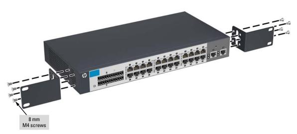
Figure 2-4. Attaching mounting brackets to the V1410-24 and V1410-24-2G Switch
