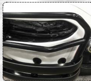
1-1/2" diameter mild steel tube
