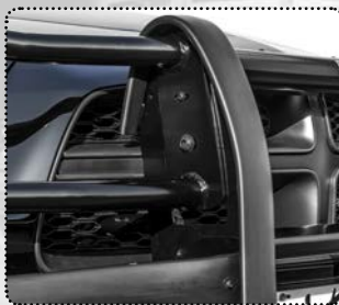
Bolts to Push Bumper with 7 gauge attachment plate
