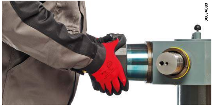
Figure 5 Touching with a taper ring gauge
