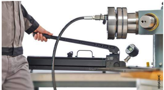
Figure 9 Hydraulic dismounting of tapered seat
