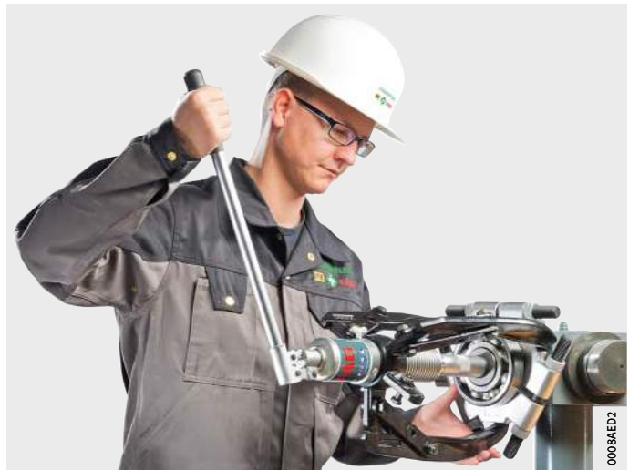
Figure 1 Dismounting by means of extraction device
