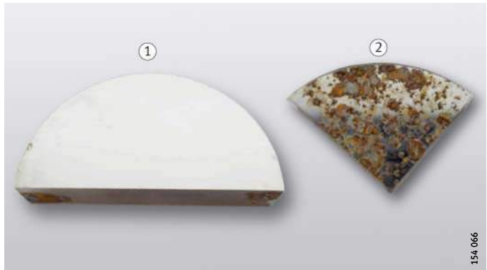
Figure 1 Corrosion resistance, comparison after 24 h salt spray test
