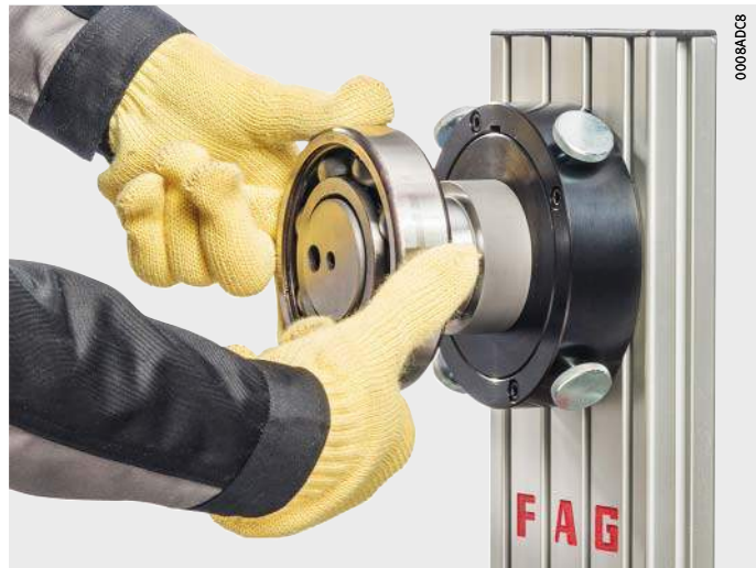
Figure 14 Sliding into place of heated bearing parts
