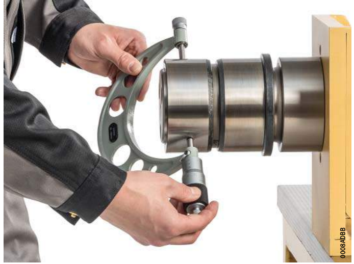
Figure 3 Measurement of expansion using external micrometer
