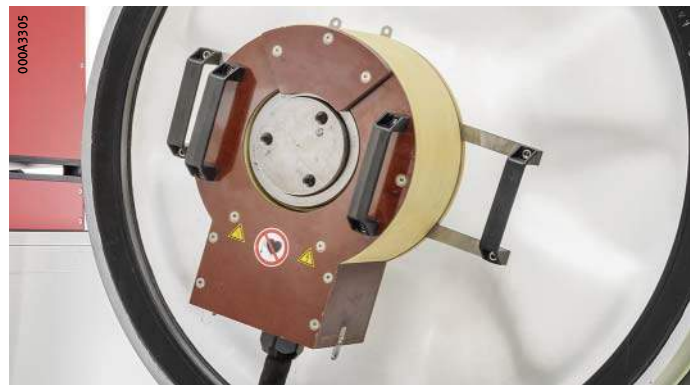
Figure 2 Rigid inductor for dismounting of wheelset bearings
