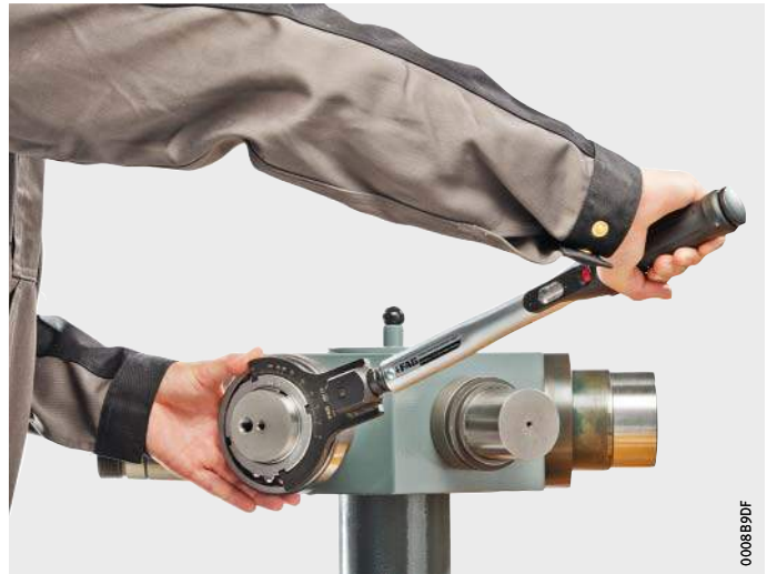
Figure 11 Mounting by means of double hook wrench
