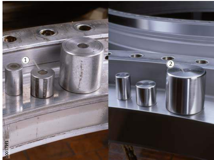
Figure 3 Rolling bearing raceway and rollers before and after reconditioning
