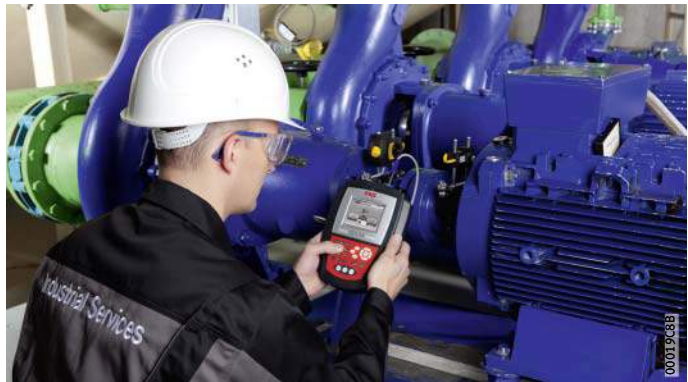
Figure 6 Shaft alignment device FAG Top-Laser EQUILIGN
