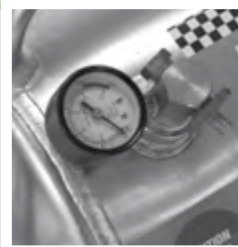
Built-in pressure gauge shows tank pressure
