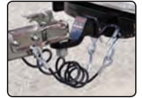
Safety cables in use
