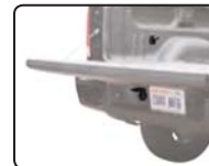
Route 7-way socket into truck bed (7')
