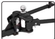
TruTrack™ WD featuring integrated sway control
