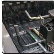
Once in rearward position, handle will self-lock into place
