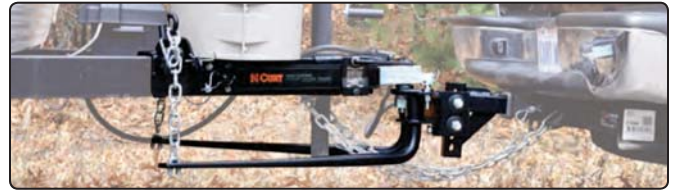
Round bar weight distribution system with sway control
