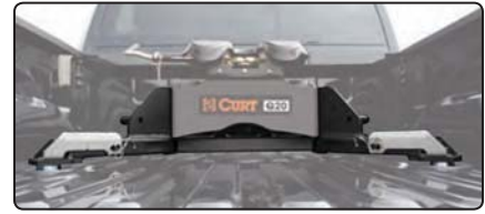
16021 Ram legs shown installed in a truck bed with 16530 Q20 head unit (16045 kit)
