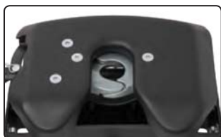
Extra wide head opening for easy coupling and high-strength interlocking jaws to eliminate noise
