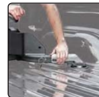
Close the anchor levers to lock the legs into place
