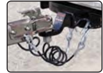
Safety cables in use
