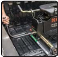
Pull handle out and angle it to the rear to release the wheels
