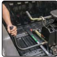
Roll unit rearward to increase trailer clearance by 12"
