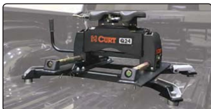
Ram OEM roller adapter legs (16022) installed in a truck bed with R24 roller (16570) and Q24 5th wheel head unit (16545)
