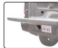
Route 7-way socket into truck bed (7')
