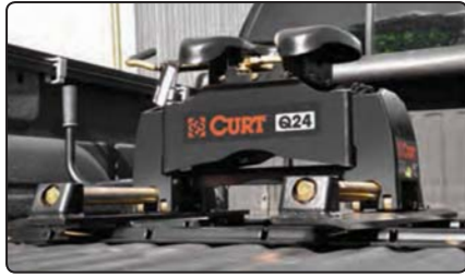
16570 R24 roller shown installed in a truck bed with 16545 Q24 head unit (16546 kit)
