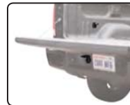
Route 7-way socket into truck bed (7')
