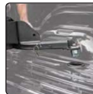
Drop the legs into the truck bed's anchoring system
