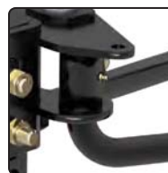
Easily accessible grease zerker fittings
