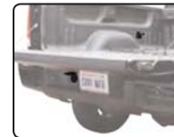
Route 7-way socket into truck bed (10')
