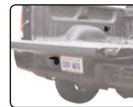
Route 7-way socket into truck bed (10')
