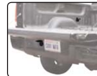
Route 7-way socket into truck bed (10')
