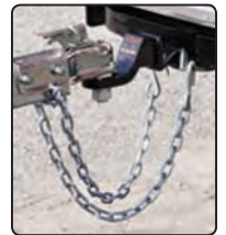
Safety chains in use
