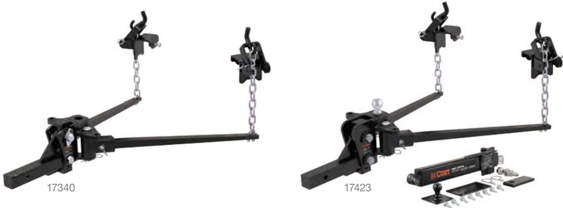
Pin-style spring bars improve strength
