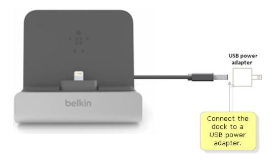
**NOTE:** You can connect the Express Dock to an AC outlet with your Apple® power supply or another USB power adapter. For a list of Belkin USB Power Adapters, click <a href="here">here</a>.
