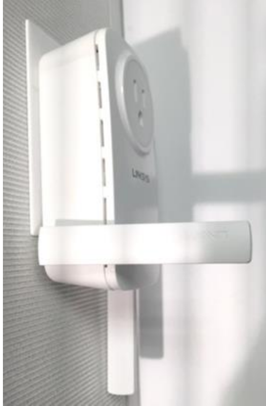
Picture A. This antenna positioning can be used if the extender is in the middle of the house.
