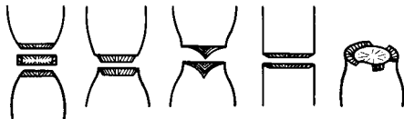
Fig. 5.1.3. Typical metal fractures in tension.
