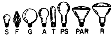
Fig. 12.5.2 Typical filament lamp shapes: S, straight; F, flame; G, globe; A, general service; T, tubular; PS, pear shape; PAR, parabolic; R, reflector.
