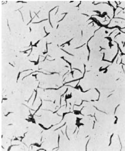
Fig. 6.3.2 Gray iron with flake graphite. Unetched, 100×.
