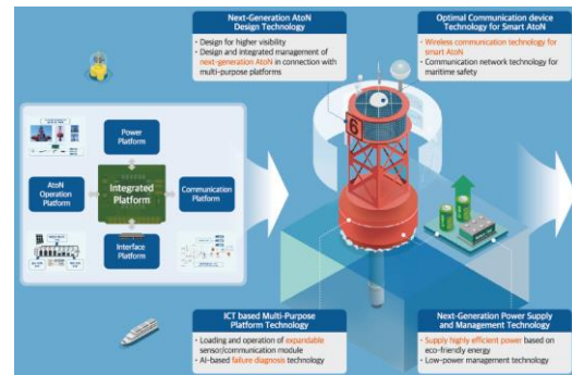
Fig. 1. Hierarchical Platform Structure of Smart AtoN
