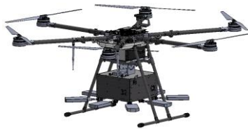
Fig. 2. Integration of Drone Systems with Communication Repeater Antennas
