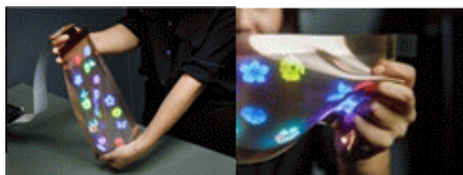
Fig. 1. Image of the Stretchable Display Prototype developed by LG Display in 2022
