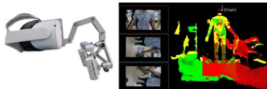
Fig. 1. RGB-D sensors on the HMD (left) and their calibrated result (right).
