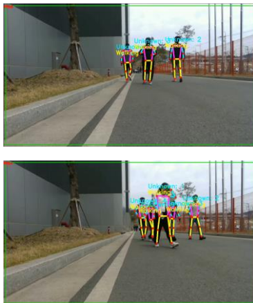
Fig. 2. Multi-Person action recognition model example
