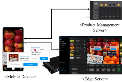
Fig. 1. Structure for product object classification based on the integration mobile device and edge server
