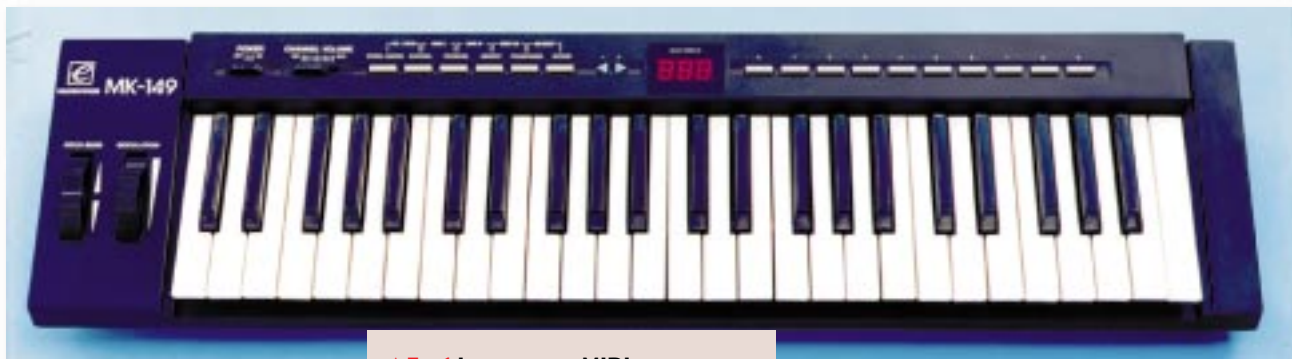
▲ FIG 1 IF YOU NEED A MIDI CONTROLLER KEYBOARD, EVOLUTION HAS FIVE PRODUCTS IN ITS RANGE STARTING FROM £35 (EX VAT). THE MK-149, SHOWN HERE, IS A FULL-SIZE FOUR-OCTAVE KEYBOARD WITH ASSIGNABLE MODULATION AND PITCH-BEND WHEELS
