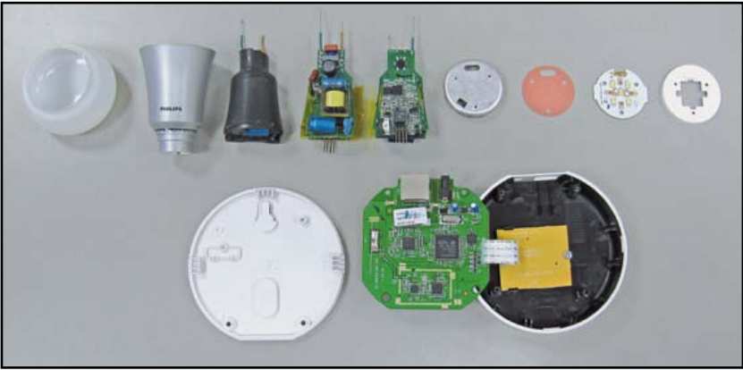
Figure 1. This is what makes hue. In the upper row the various components that make up the bulb; below, the Bridge.
