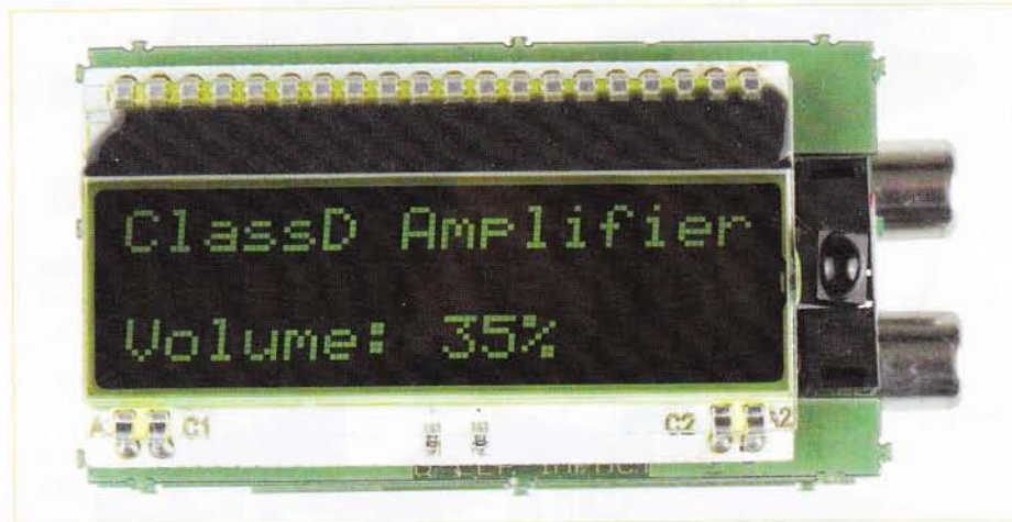
Figure 10. The volume setting is shown around five seconds after the welcome message. Other settings are shown below.
