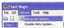
Figure 5. Options -> Advanced Options...: Checking this box enables Flash Magic to put the Sceptre in programming mode and reboot without your having to do anything.
