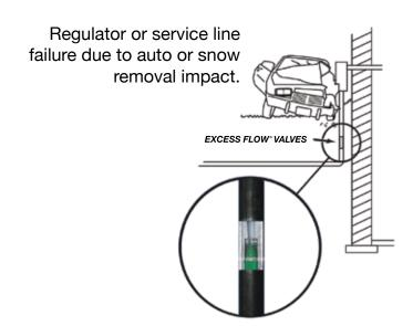
The GasBreaker AutoCock™ Excess Flow® Valve is designed for installation under live gas condition, pressures up to 150 psig, in existing steel gas utility service lines or risers immediately upstream of the meter set. Auto-Cocks protect against unsafe conditions that result from damage to the exposed or aboveground portion of the service line.
