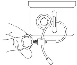
4. To permanently lock the Cable Lock, either grasp the lock body with pliers and turn set bolt with a wrench until the bolt head breaks off or, twist the bolt head with your fingers until it breaks off.
