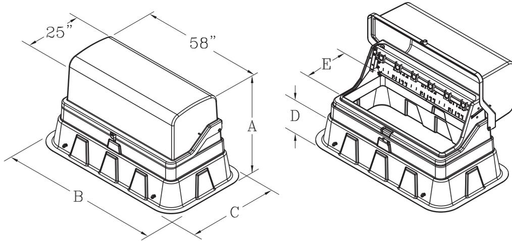
All mounting plates are fully adjustable from 0°-25°. Detents exist for 0°, 5°, 12°, 20° and 25°. This unit does not accommodate 200 Amp taps off 600 Amp service.
